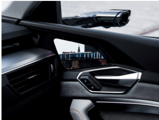
Figure 2.4: A practical example of the Mirror View project designed by Audi
