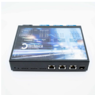
Figure 3.5: MediaGateway from Technica Engineering
