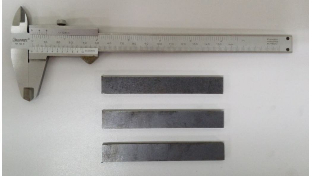
Figure 3.1. Steel beams specimens.
