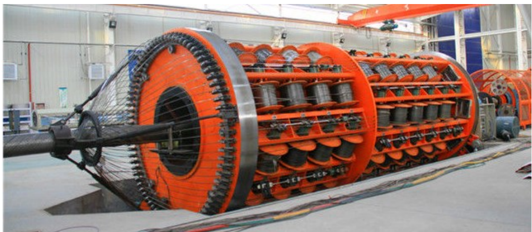
Figure 2.6. Tensile armor machine [20].
