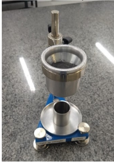
Figure 21 – Powder mixture fails to flow in Hall and Carney funnels.
