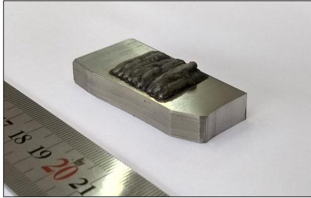
Figure 35 – Irregular layers achieved after overlay deposition of bead 44
