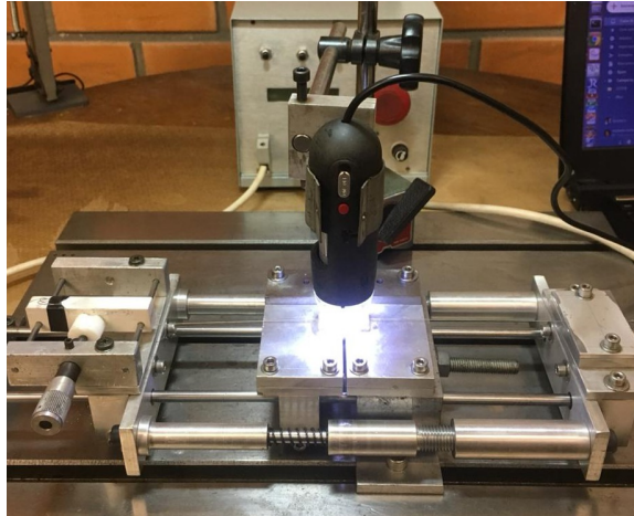
Figure 31: Microscope positioning over the inserts.
