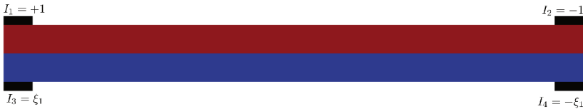
Figure 28 Experimental configuration for EIT with two plies and four electrodes (Example 4).
