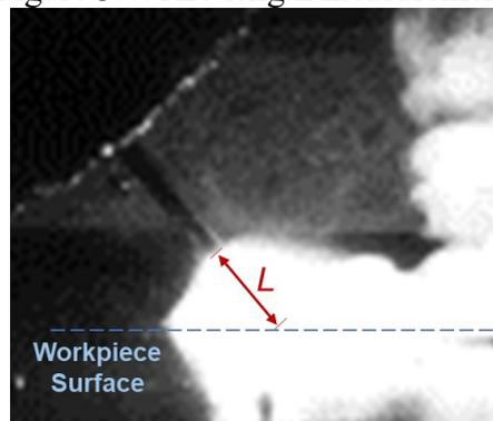
Turbulence and other visible features on the forward and backward plasma jets (the plasma jet within the arc was not measured) were used to track the jets speed and direction,
