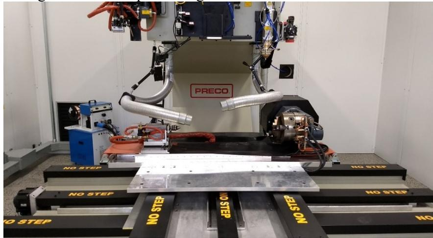
The moving system has a XY-table with **10 m/min** maximum feed rate. The laser welding head moves in the Z-axis. The last two axis are given by a rotary tilting table attached to the XY-table, but it was not used for the present work.
