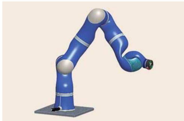
Figura 6 – Robô industrial com 7 DOFs.
