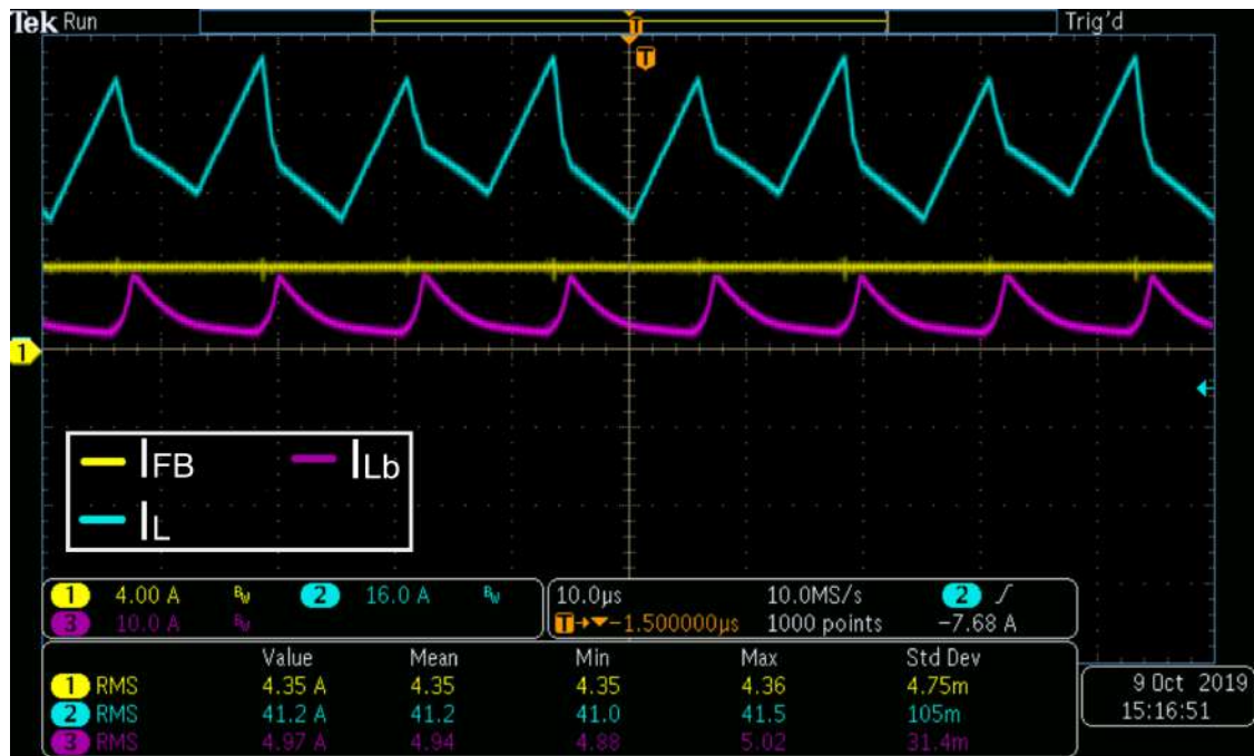
Figure 134 – Current in the Full-bridge Stage, Push-Pull Stage and Buck converter for the negative power flow
