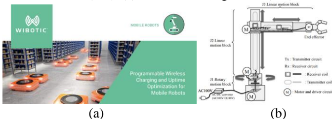
Figure 3.4 – Industry and Robotic examples: (a) Autonomous robots from WiBotic (IPT), (b) Robot arm configuration (IPT).
