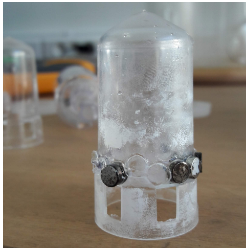
Figure 4.12: Destroyed CO 2 sensor
