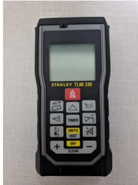
Figura 19 – Trena laser Stanley TLM 330
