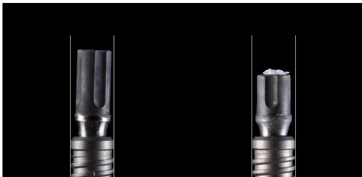
Figure 10. Long titanium base (left) with apparent permanent deformation consecutive to loading/fracture. Apparently intact short titanium base after loading/fracture.
