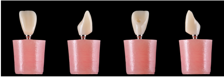
Figure 5. Buccal, mesial, lingual and distal view of experimental BSRC before closing of fastening hole with composite resin.
