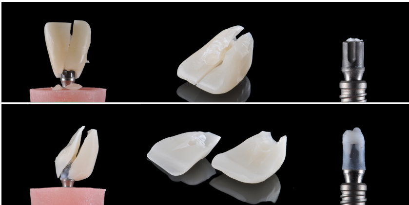
Figure 11. Emax BSRC with typical buccolingual fracture and clean titanium base surface (top). Shofu BSRC with a typical mesiodistal fracture and remaining luting composite onto the titanium base (bottom).
