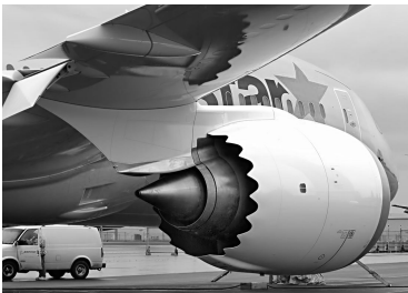
Figure 1.7 – Underwing mounted turbofan engine. Source: <www.aircraftnerds.com>.
