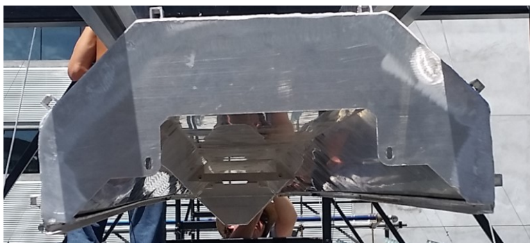
Figure 3.3 - Front view of the trapezoidal cavity receiver without the absorber element.
