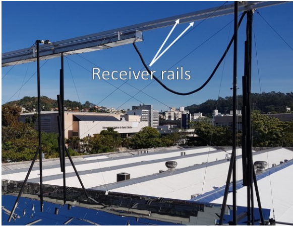
Figure 3.4 - Fixation of the receiver on rails.
