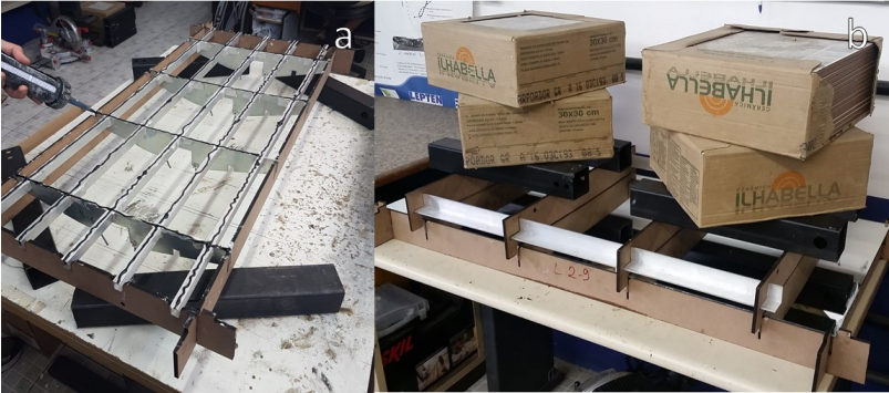
Figure B- 3– Fixation of the mirror. a) Application of glue on the modular structure supported by the MDF template in order to fixate the mirror. b) weights pressing the mirror against the modular structure.
