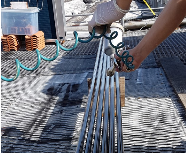
Figure B- 8 - Painting of the absorber tubes.
