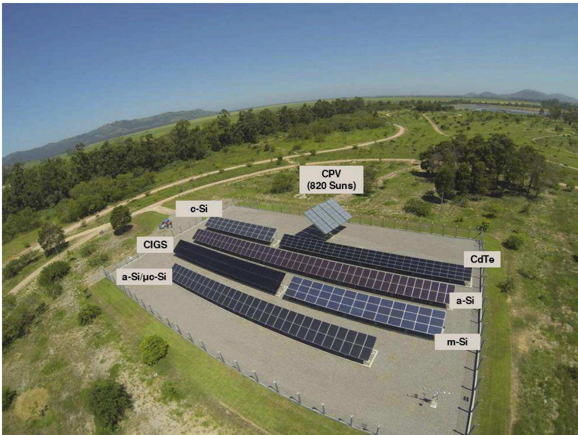
Figure 24 - Aerial view of one (ES # Capivari de Baixo-SC, 28°S, 48°W) of the eight identical R&D ESs, with approximately 54 kWp of fixed, latitude-tilt PV.
