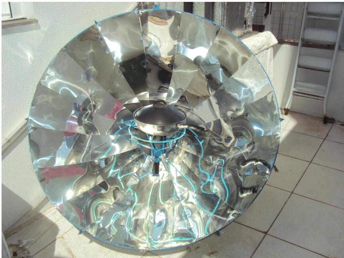
**Figure 4 A parabolic solar cooker – source: the authors**
