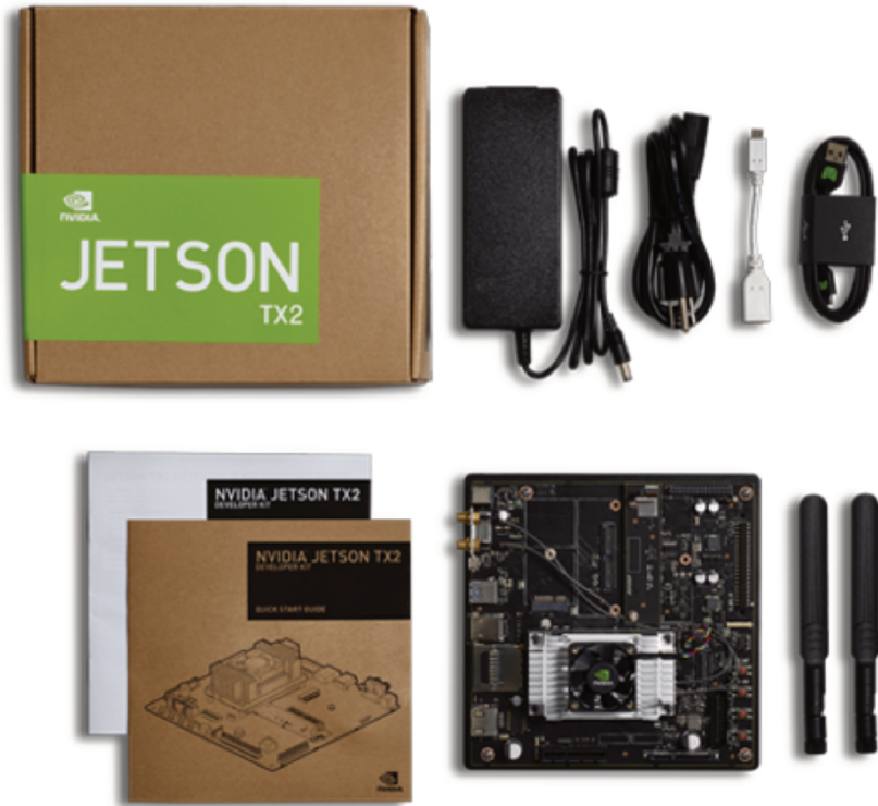
Figure 6.3: Jetson TX2 Development kit and accessories
