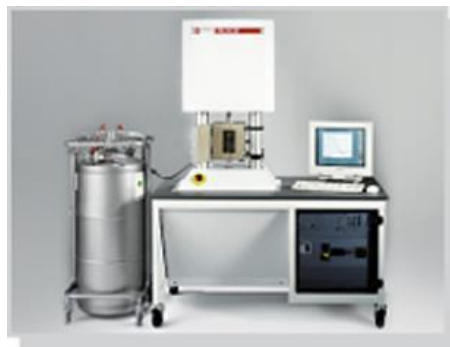
Figure 33 – Gabo Eplexor 500N DMA machine utilized for DMA measuring
