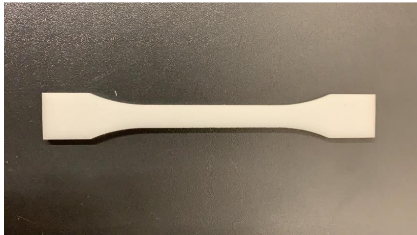
Figure 30 – Tensile testing specimen machined following DIN EN ISO 527-2 Type B
