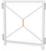
Figure 2 – Example of a vertical planar cable-driven robot structure. Source: Adapted from (BRUCKMANN et al., 2008).
