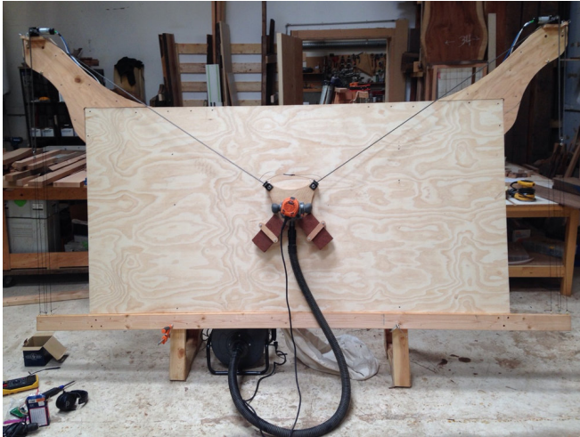
Figure 26: Planar Cable Driven Robot for cutting wood - Maslow CNC. Available at Maslow (2018).
