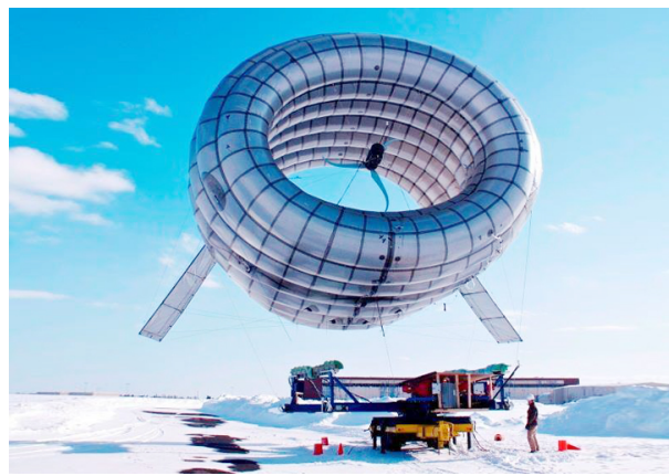
Figure 2.1: Static aerogenerator constructed by Altaeros Energies [1].
