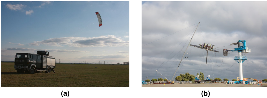
Figure 2.2: AWES based in (b) drag forces and (a) lift forces.
