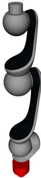
Figure 9 – LWA4P extended arm.
