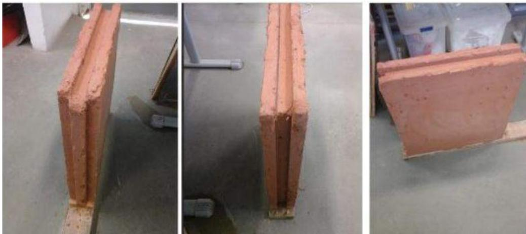
Figura 14: painel de trama de bambu e garrafas pet no interior e argamassa calfitice.
