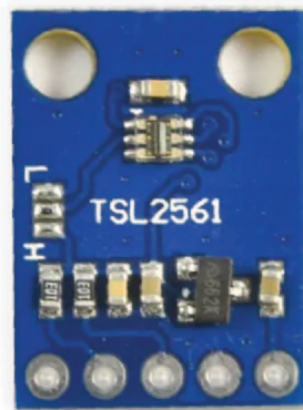
Figure 18 – Light-to-digital converter TSL2561. Height = 2cm.
