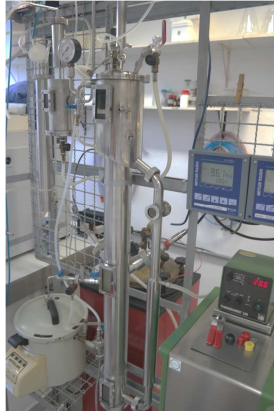
Figure2- Overview of the 5L airlift bioreactor used in this study.
