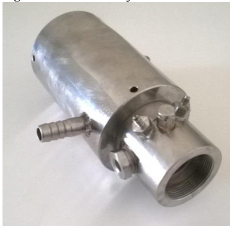
Figure 12. Detail of the jacketed cell made of stainless steel.
