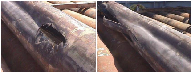
Figure 1.2 – 0.4064 m (16 in) outer diameter casing collapsed during hot fluid circulation due to APB (PATTILLO et al. , 2006).
