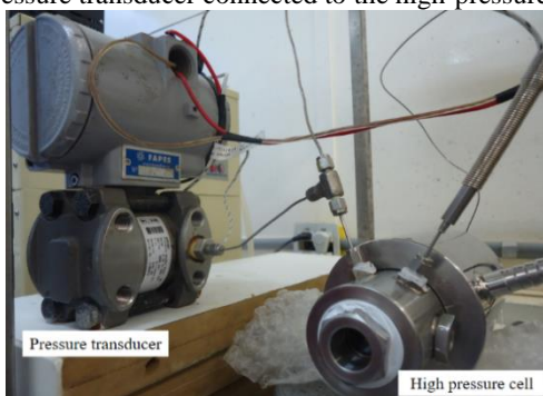
Figure A.12. Pressure transducer connected to the high-pressure cell.
