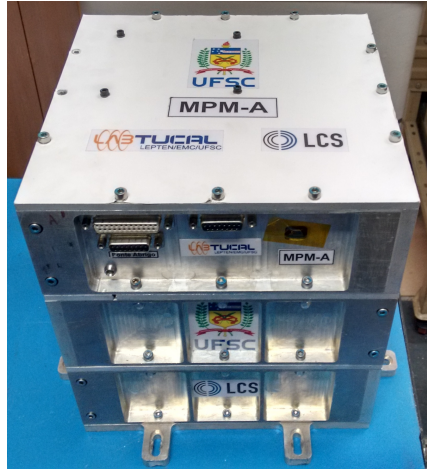
Figure 88: MPM-A instrument after acceptance tests - ready for flight
