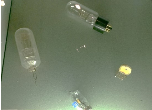
Figure 1.1 – Quartz crystal resonators from 1960's. Picture taken at the Musée du Temps in Besançon, France.
