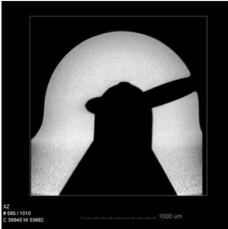
Figure 20. Tomogram of injector nozzle used in the diesel engine (LMPT/UFSC).
