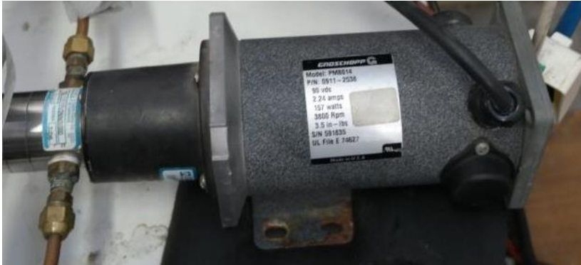
Figure 37: Picture of the pump coupled to the electrical motor
