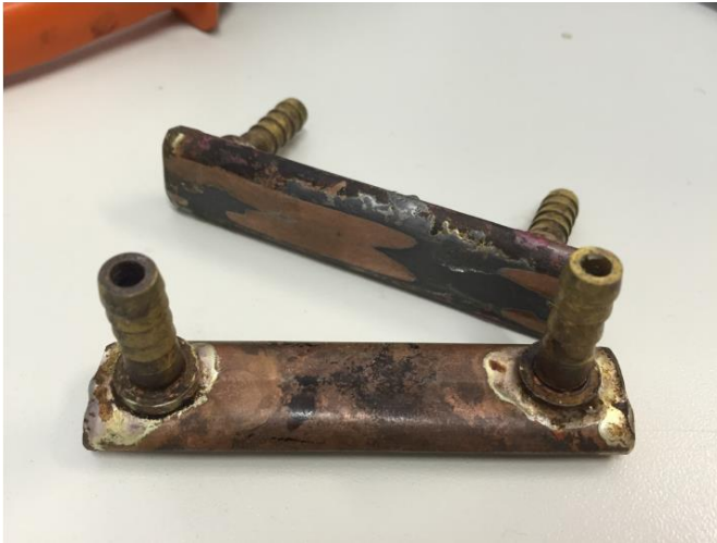
Figure 38: Overview of the heat sink
