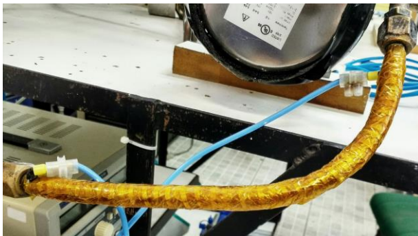
Figure 27: Picture of the superheater
