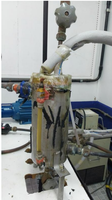
Figure 35: Picture of the post condenser
