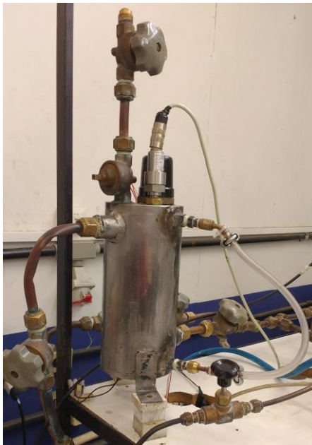
Figure 26: Picture of the boiler
