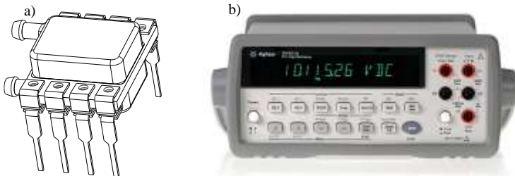
Figure 5.10 – a) Honeywell pressure transducer; b) Agilent 34401A DMM.
