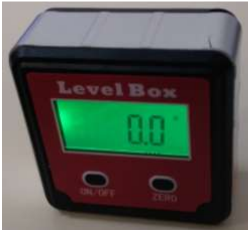
Figure 5.17 – Digital inclinometer XB-90 used in this work.
