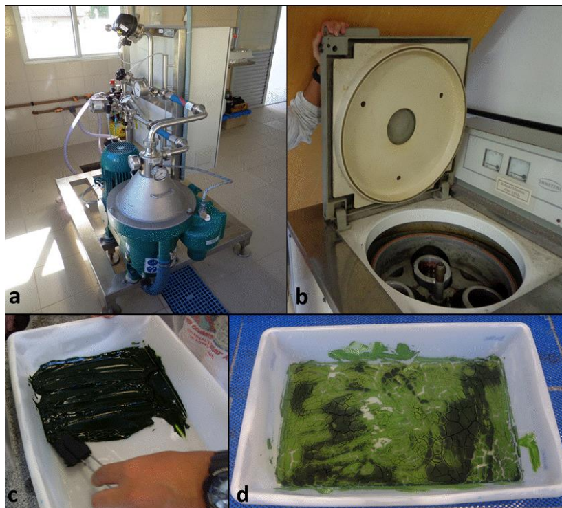
Figure A4 Centrifuges used to harvest the microalgae biomass. (a) continuous centrifuge (b) batch centrifuge. Obtained biomass. (c) wet paste spread in thin layer, (d) dried biomass.
