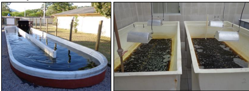
Figure 2.2 Open systems for microalgae cultivation. Raceway pond (left) and open tanks (right), both located at Laboratório de Cultivo de Algas (LCA), Florianópolis - SC, Brazil.
