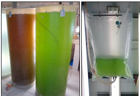
Figure 2.3 Closed systems (PBRs) used for microalgae cultivation. Horizontal tubular PBR (left), located at Laboratório de Cultivo de Algas, Florianópolis – SC, Brazil and bag system (right), located at Solar Biofuel Research Centre, Brisbane – QL, Australia.
