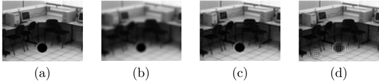
Figure 8 – Reconstruction results for a video sequence containing an outlier (taken from (ZIBETTI; MAYER, 2007)). (a) Original image (HR). (b) Bicubic interpolation. (c) Single frame based SRR. (d) L_2 norm based SRR with the Borman and Stevenson (BORMAN; STEVENSON, 1999) method.
