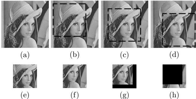
Figure 6 – Illustration of border effect innovations for global translational motion (taken from (COSTA, 2007)). (a) Original scene. (b)-(d) HR images in time instants t - 2 , t - 1 and t (dashed) relative to the scene. (e) \mathbf{x}(t - 1) . (f) \mathbf{x}(t) . (g) Registered image \mathbf{G}(t)\mathbf{x}(t - 1) , considering Dirichlet boundary condition. (h) Innovations \mathbf{s}(t) .
