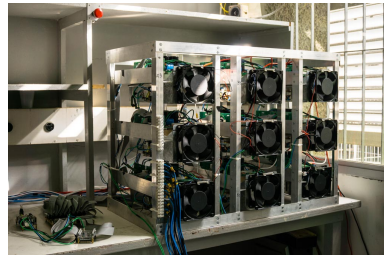
Fig. 4. Photograph of the prototype. Cage with height of 60 cm, depth of 41 cm and width of 83 cm.
