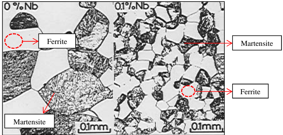
Figure 3.33 - Effect of Nb on the grain size of dual-phase steel maintained at 1100 °C for 100 h.
