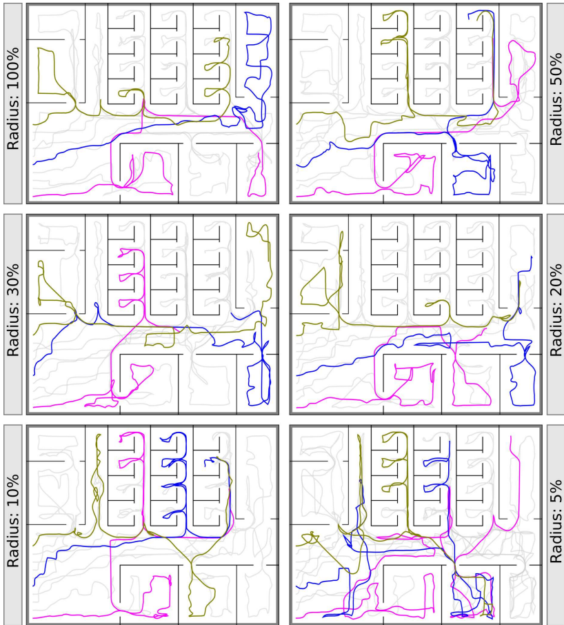
Figure 37 – Paths of robots in office-like workspace for different communication radiuses.
