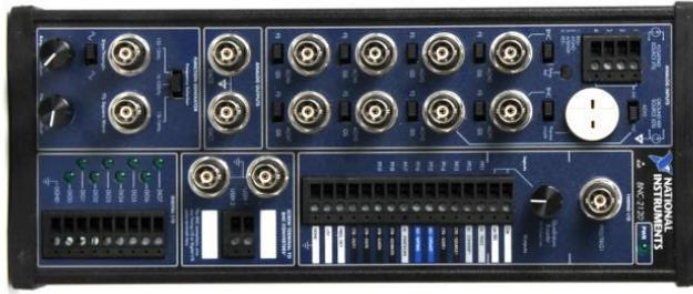
Figure 16: BNC 2120 I/O board
