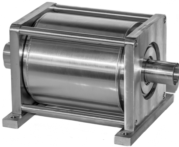
Figure A.7 – Nested Halbach Cylinder magnetic circuit built according to the dimensions obtained from the proposed design procedure.
