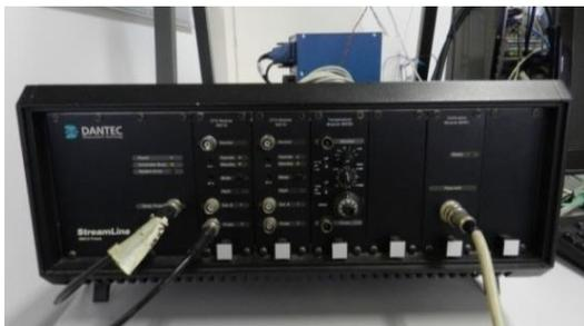
Figura 32: *Chassis* central (*StreamLine*).
