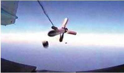
Figure 7 Deployed fibre optic towed decoy.
