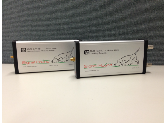
Figura C.2: Módulos Signal Hound, transmissor USB-TG44A e receptor USB-SA44B.
