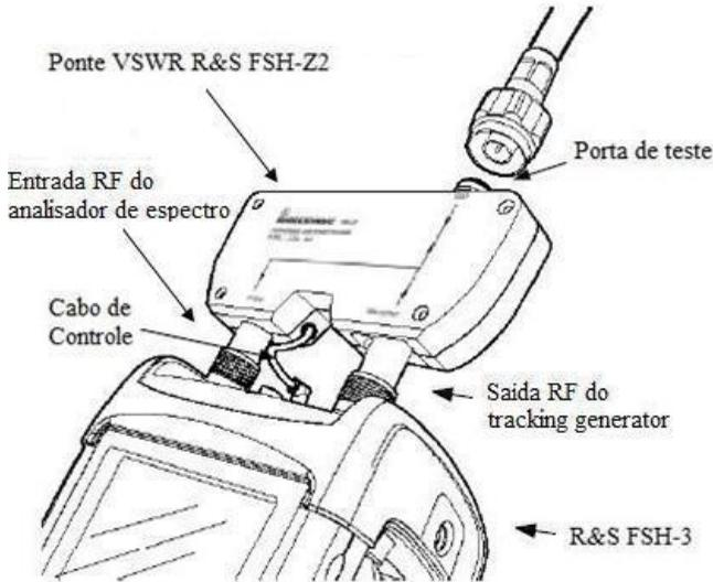
Figura 18: R&S FSH-3 com a Ponte VSWR R&S FSH-Z2 [43].
