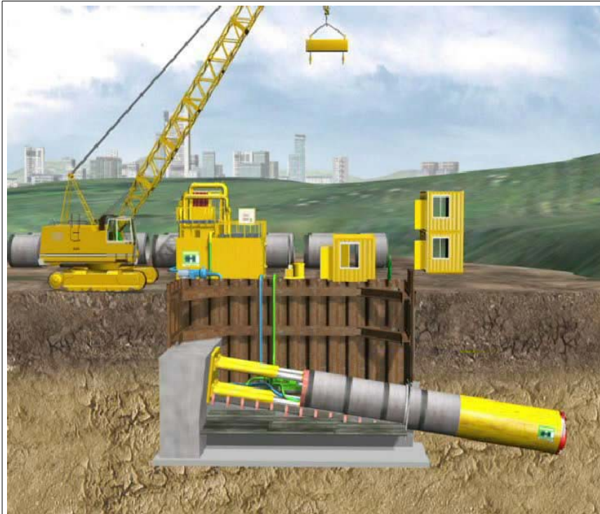
Figura 3.20: Emboque do Shield
