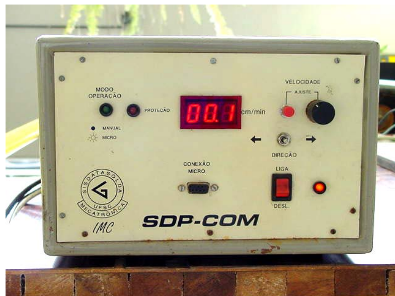
Figura 2.17 – Painel frontal do gabinete de controle do “SDP”.
