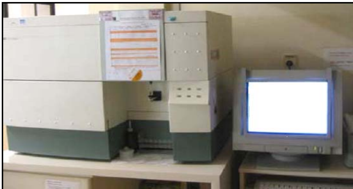
FIGURA 7. Citômetro de fluxo, modelo FACSCallibur ( Becton Dickinson Immunocytometry Systems, San Jose, CA, U.S.A. ).
