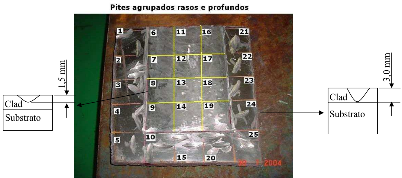
Figura 3.10: Corpos de prova de 1, 2, 3, 4, 5, 10, 15, 20, 21, 22, 23, 24, 25 agrupados rasos e 6, 7, 8, 9, 11, 12, 13, 14, 16, 17, 18, 19 simulando pites agrupados profundos.
