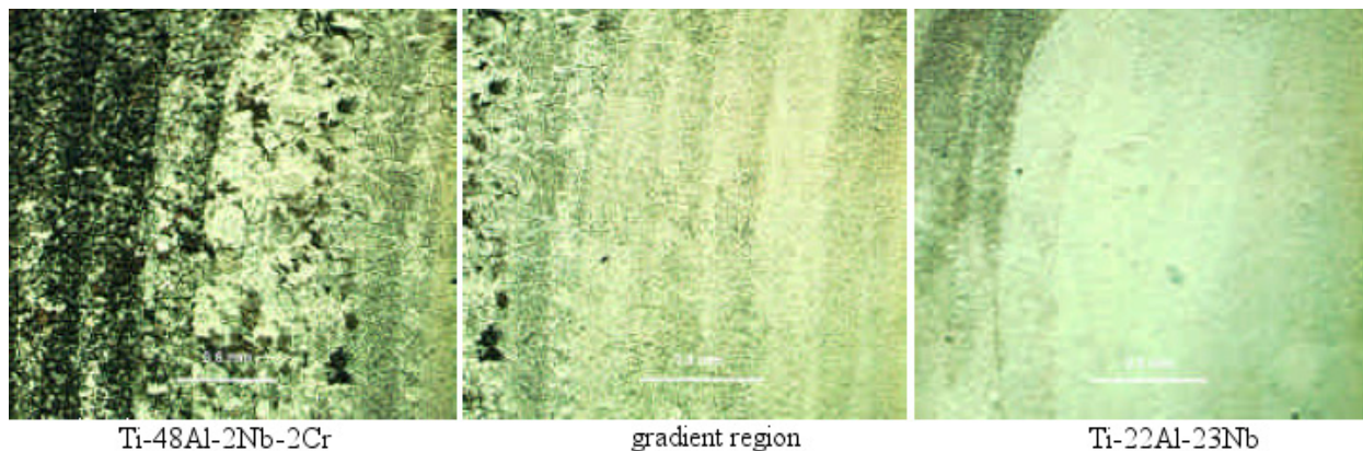
Figure 2-14. Different graded transitions of aluminium alloys obtained by LENS™ process (Chavez, 2000).
