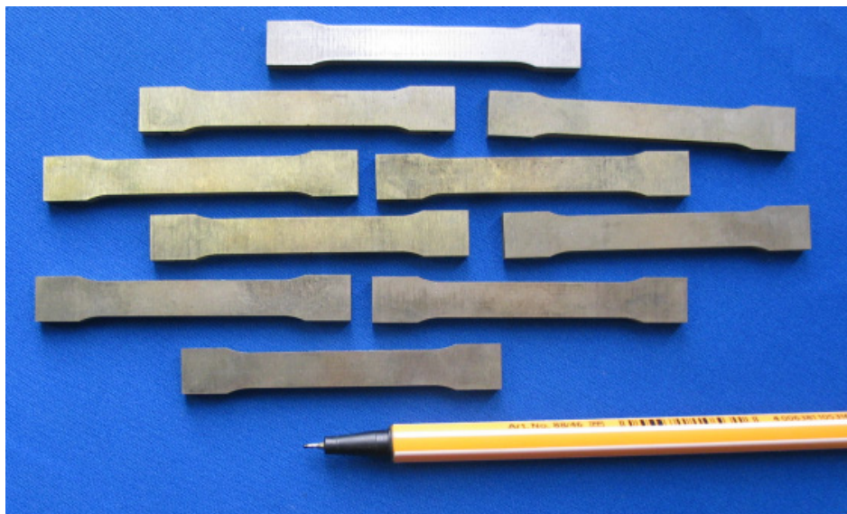
Figure 7-25. Tensile test specimens after final wire spark erosion.
