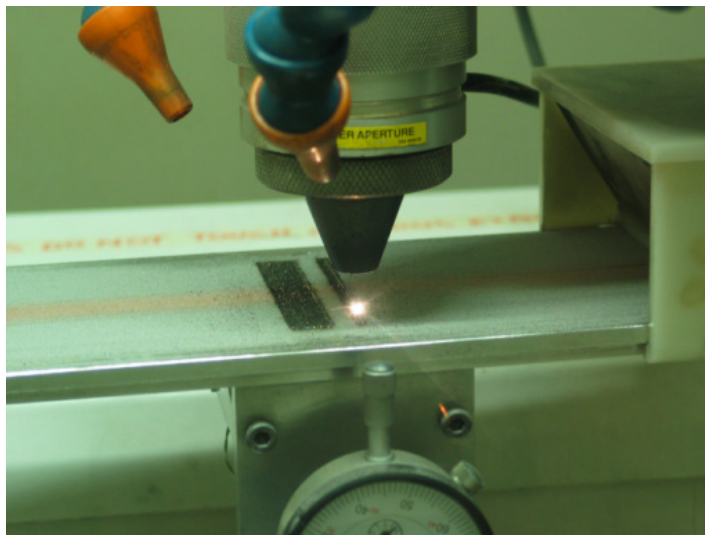
Figure 7-22. Photograph of the manufacturing of a layer for two specimens.
