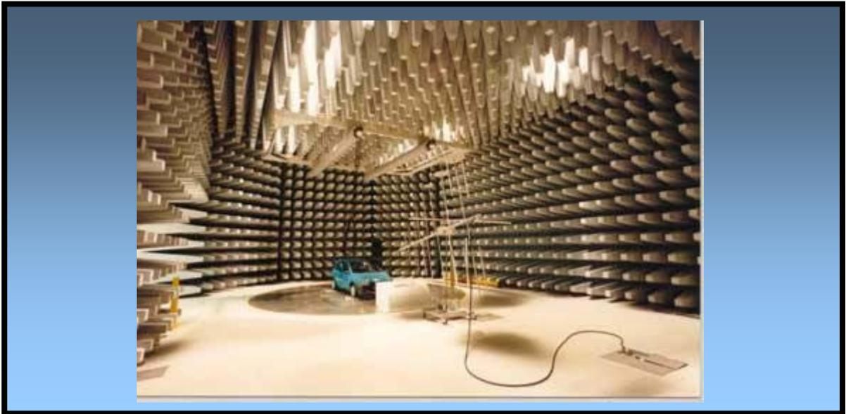
FIGURA 4.4 – UMA CÂMARA SEMI-ANECÓICA DA ETS-LINDGREN
